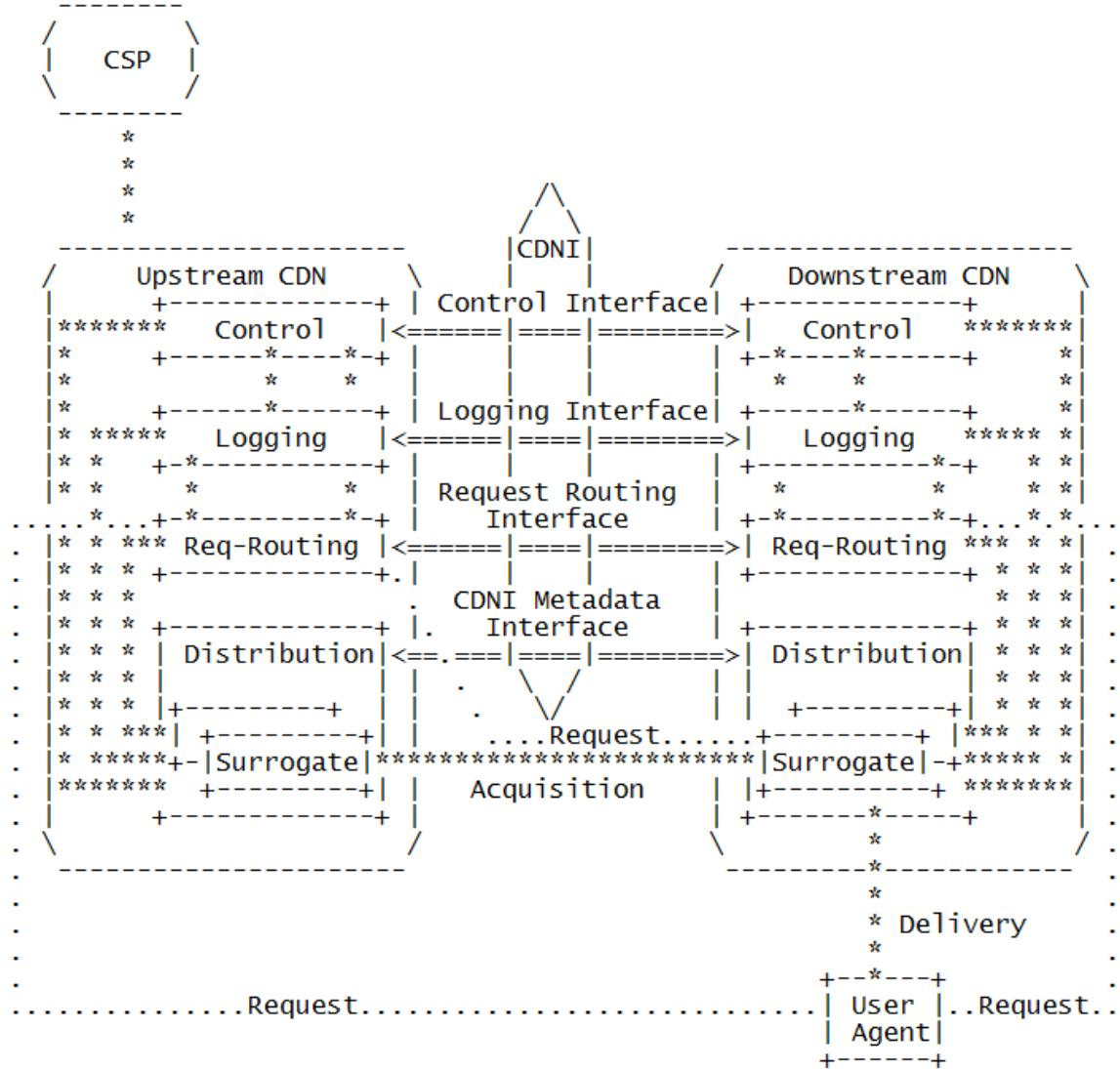
Figure 1: CDNI Model and CDNI Interfaces
