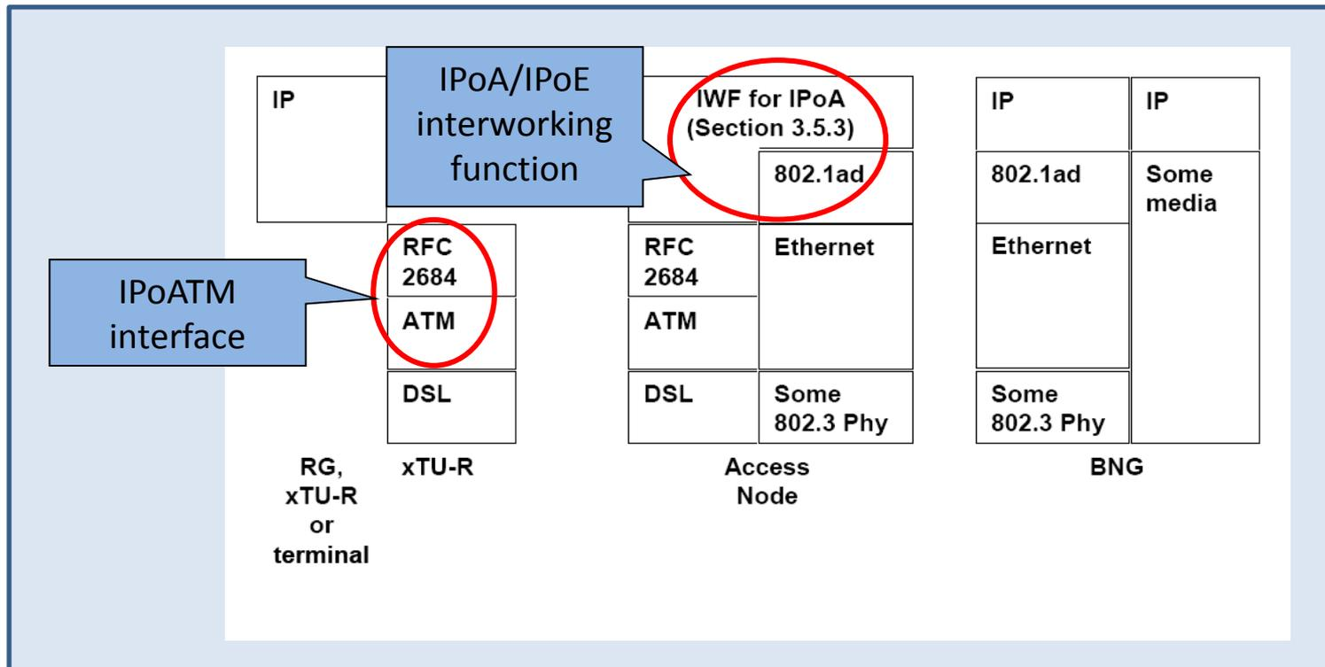
Figure: End-to-end protocol processing for IPoA access
