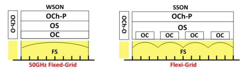
OCh-P: OCh Payload, OCh-O: OCh Overhead, OS: Optical Signal, OC: Optical Carrier, FS: Frequency Slot
