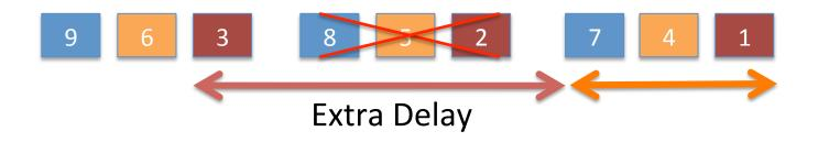
Interleaving sends data out-of-order, can recover from bursty loss
