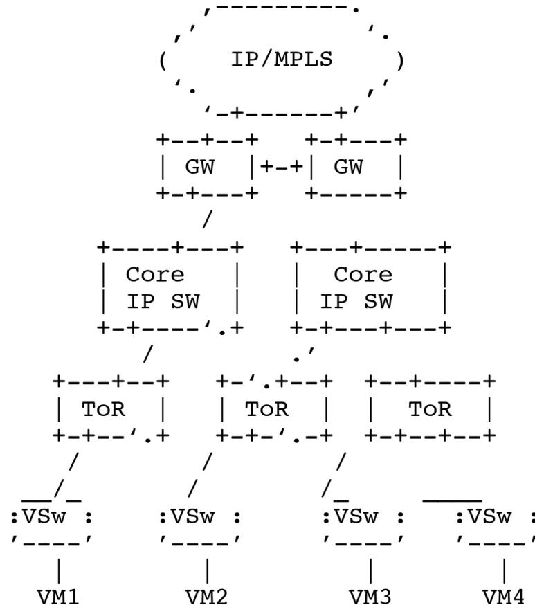
Figure 1: A typical DC network
