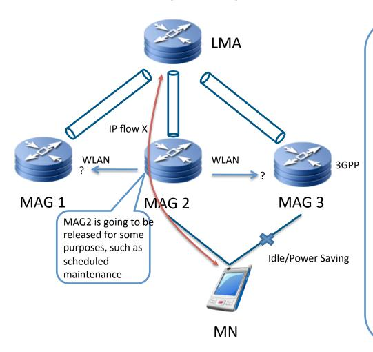
1. the LMA can either to switch the IP flow x to the 3GPP access, or to switch the flows to another WLAN access (if available). 2, if 3GPP access is currently in Idle mode, the LMA may switch the IP flow X to MAG 1 according to the MN status information and other policies, rather than wake up the 3GPP access; 3, the LMA may also switch the IP flow x to MAG 3 after waking the 3GPP access up, if the radio quality of WLAN access on MAG 1 is not good enough.
