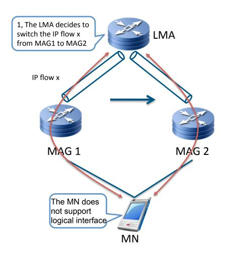
•PMIPv6 IP flow mobility solution requires logical interface capabilities on the MN
