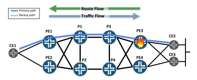
Requires protecting service (or LSP) endpoint on primary node (PE3)
