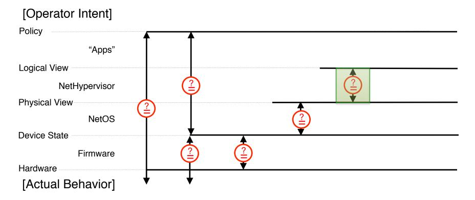
RIB == FIB? Compare device state against the actual bits and bytes in TCAMs, etc.
