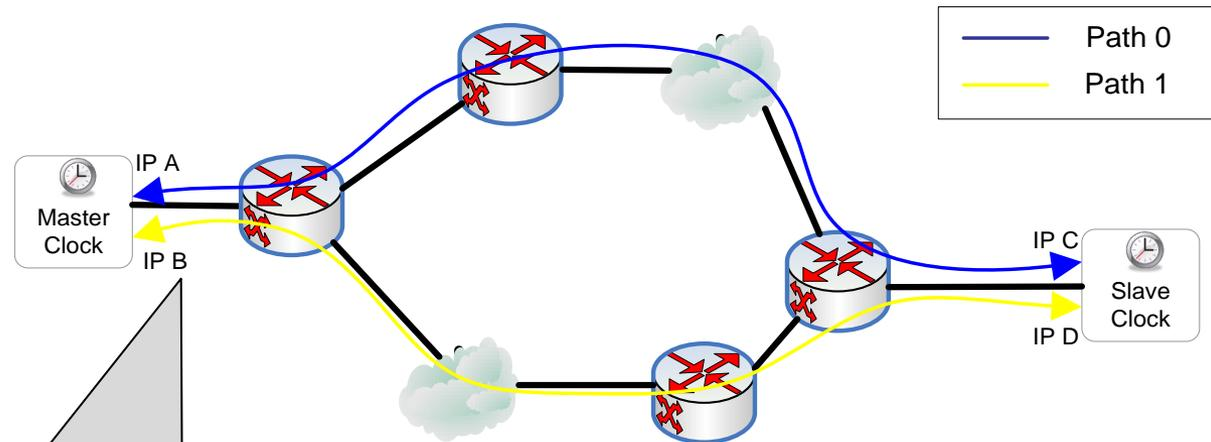
Master / slave use {master IP, slave IP} pairs to identify path ID.
