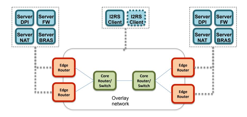
The Server DPI(FW, NAT) is located in the application model in the I2RS structure
