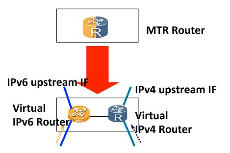
For illustration, two virtual Routers are used to represent MTR Routers
