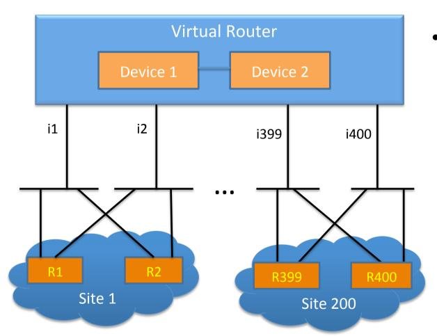
The network using virtual router which operate multiple physical devices as logically one, e.g. IRF of HP, more networks can be plugged in, accordingly the number of IS-IS neighbors probably beyond 255
