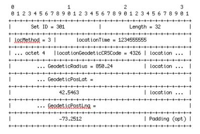
Figure 4: Data record of a circle-based geodetic location
