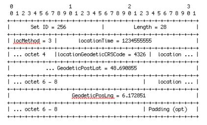
Figure 2: Data record of a geodetic 2D point location
