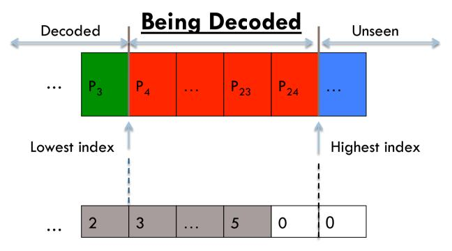
Any linear combination of packets with indices < Highest index will help decoding
