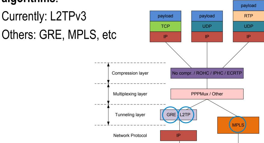
Backwards compatibility with TCRTP (RFC4170, payloa implemented in some places), **RTP** payload payload which would become one of UDP **TCP UDP** the TCM-TF options No compr. / ROHC / IPHC / ECRTP Compression layer PPPMux / Other Multiplexing layer Tunneling layer GRE / L27P **MPLS** Network Protocol
