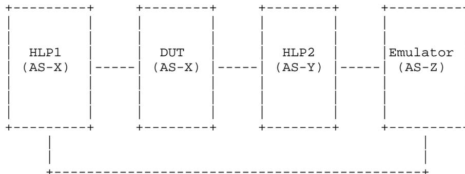
Figure 4 Four Node Setup for EBGP and IBGP Convergence
