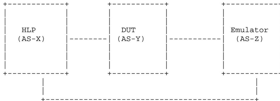
Figure 2 Three Node Setup for eBGP and iBGP Convergence
