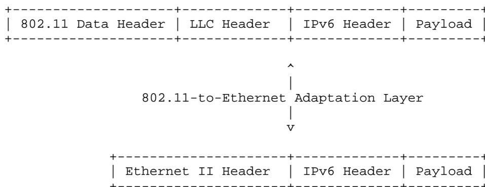
The Receiver and Transmitter Address fields in the 802.11 Data Header contain the same values as the Destination and the Source Address fields in the Ethernet II Header, respectively. The value of the Type field in the LLC Header is the same as the value of the Type field in the Ethernet II Header. The other fields in the Data and LLC Headers are not used by the IPv6 stack.
