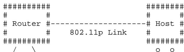
During several capture operations running from a few moments to several hours, no message relevant to the BSSID contexts were captured (no Association Request/Response, Authentication Req/Resp, Beacon). This shows that the operation of 802.11p is outside the context of a BSSID.
