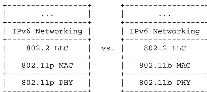
But, there are several deployment considerations to optimize the performances of running IPv6 over 802.11p (e.g. in the case of handovers between 802.11p Access Points, or the consideration of using the IP security layer).
