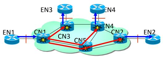
E.g., packet over TDM network, and CN1 has the packet multicast capability
