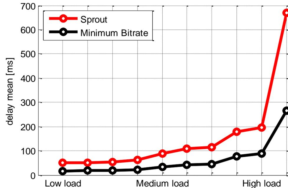
Sprout is not behaving well in simulated LTE environment
