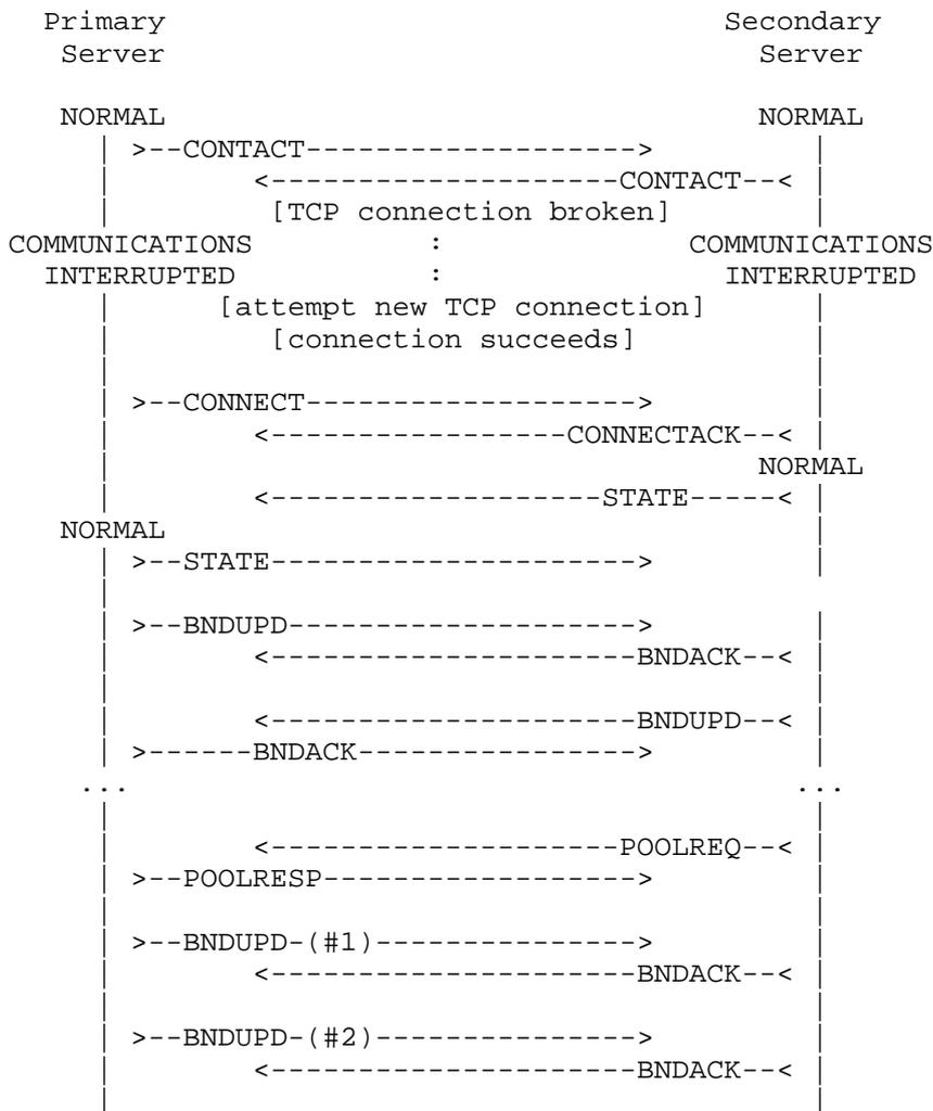
Figure 6: Transition from NORMAL to COMMUNICATIONS-INTERRUPTED and back (example with 2 addresses allocated to secondary)
