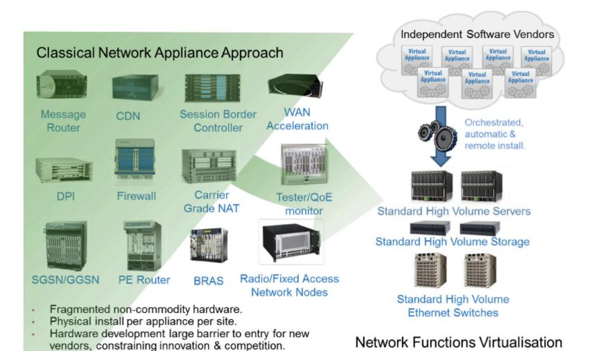
Figure 1: Vision for Network Functions Virtualisation
