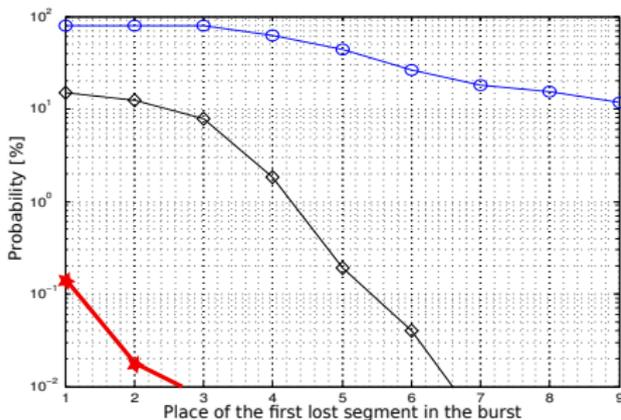
**Probability for 1, 2 or 3 segments of the burst to be correctly transmitted when one of the previous segment of the burst has been lost**
