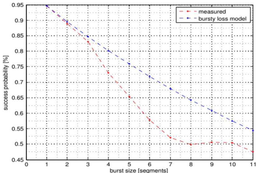
Burst consequences according to the model and real experimentations
