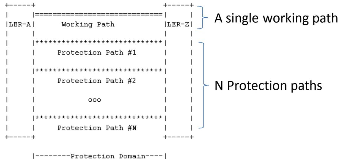
Example of multi-failure protection
