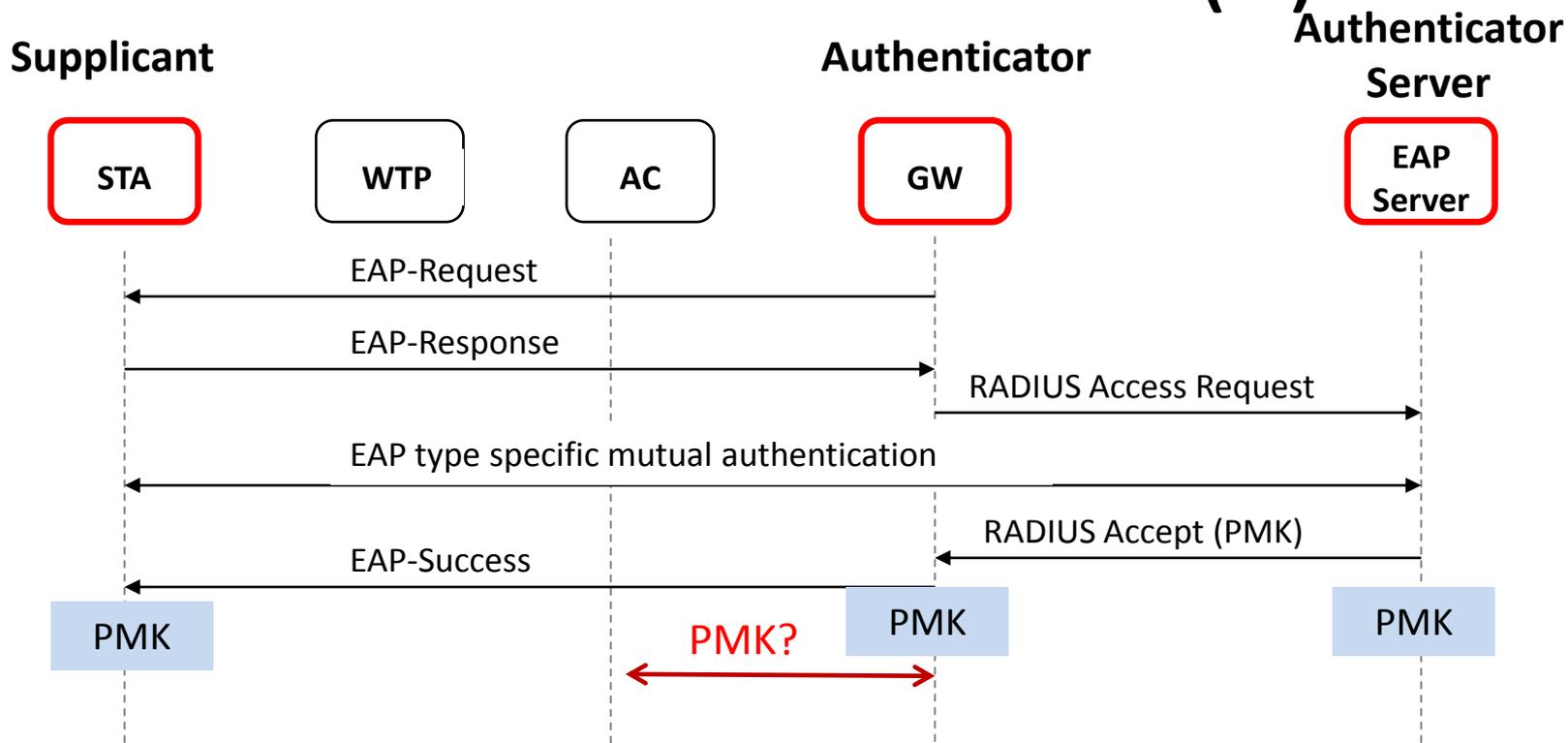
In a WLAN network, when a STA tries to connect to the WTP, mutual authentication with a EAP server is needed.
