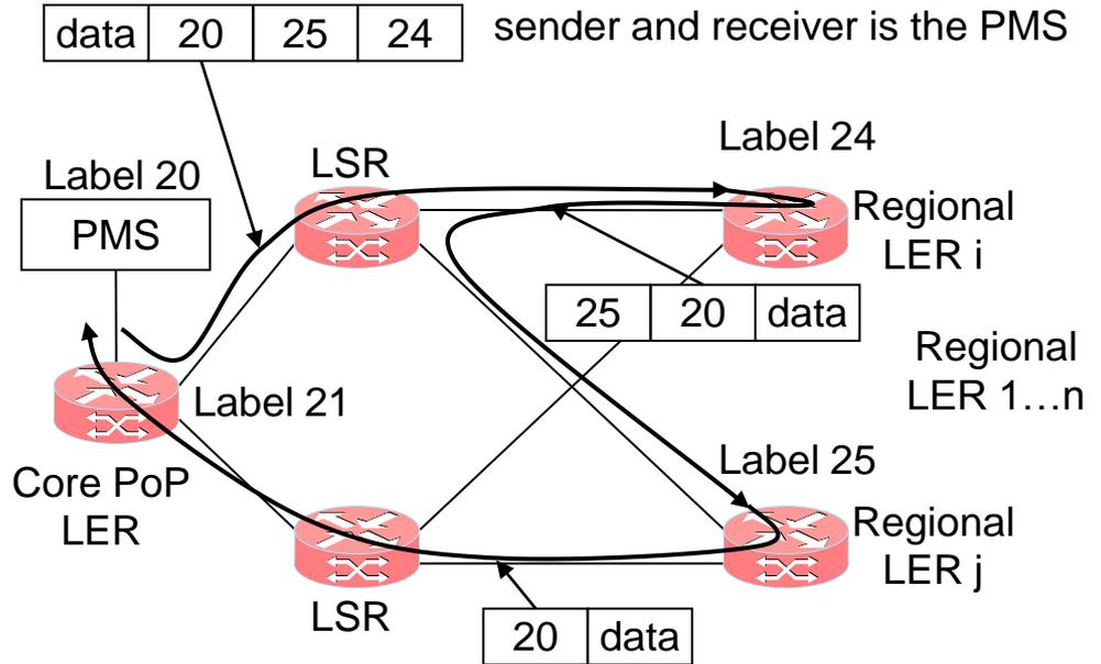
→ PMS based LSP measurement, here with 3 LSP segments
