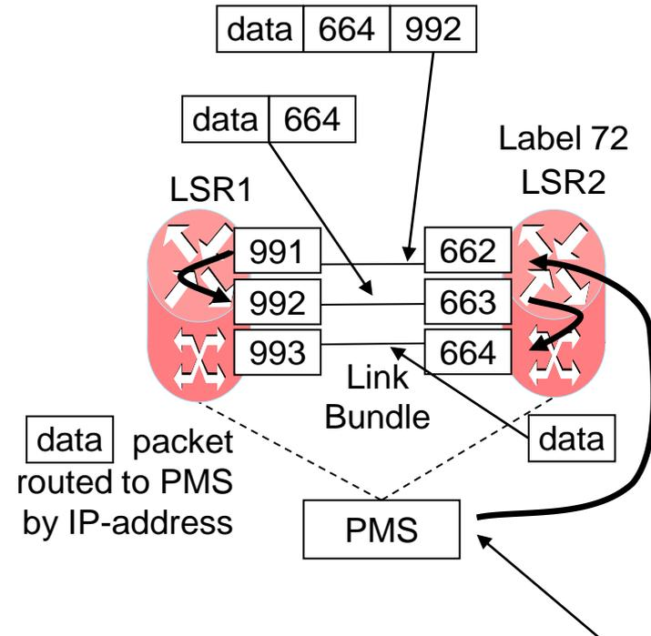
Example of a measurement packet, sender and receiver is the PMS
