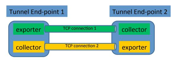
The scenario that two TCP connections are established between two tunnel end-point, each connection for one direction. There will be an exporter and a collector process on each tunnel end-point.
