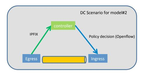
IPFIX is primarily used to convey Information about IP flows passing through a network element (extend to convey tunnel congestion):
