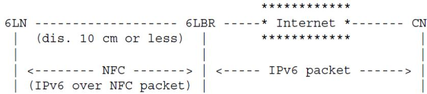
Figure 5: NFC-enabled device network connected to the Internet
