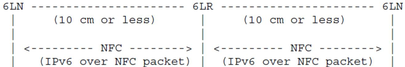
Figure 6: Isolated NFC-enabled device network
