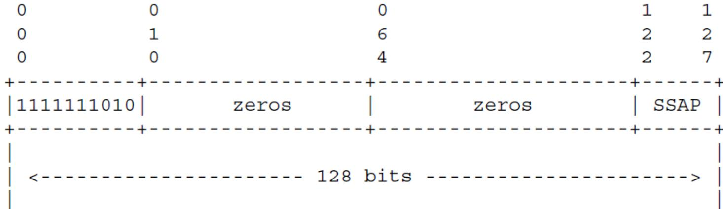
Figure 4: IPv6 link-local address in NFC
