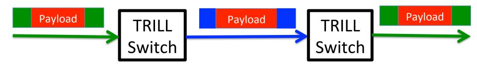
Forwarding a TRILL Data packet from a green technology link to a blue technology link and back.
