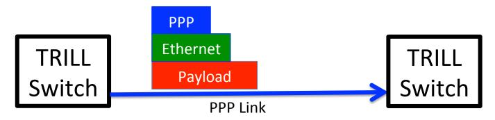
• But the extra Ethernet header you have stuck in is useless. It gets thrown away, along with the PPP Header, at the destination TRILL switch port. If the PPP source port has no address, you have to make up fake MAC addresses to put in the useless Ethernet header.
