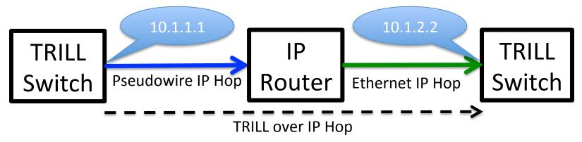
Each IP hop composing the TRILL hop is over some lower layer, possibly different for each hop, and all irrelevant to TRILL.
