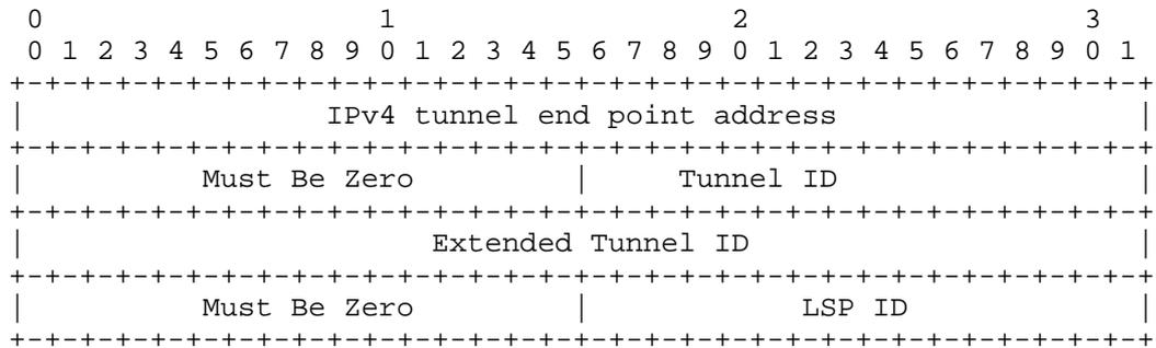
The IPv4 tunnel end point address, Tunnel ID, Extended Tunnel ID and LSP ID are as defined in [RFC3209].
