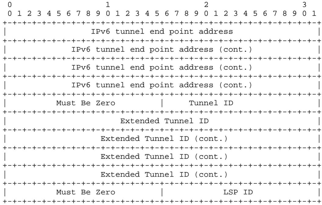
The IPv6 tunnel end point address, Tunnel ID, IPv6 Extended Tunnel ID and LSP ID are as defined in [RFC3209].
