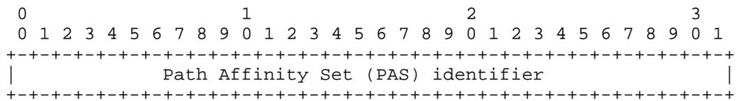
The Path affinity Set (PAS) identifier is a single number that represents a summarized SRLG for the reference path against which diversity is desired. The node identified by the "IPv4 Diversity Identifier source address" field of the diversity XRO subobject assigns the PAS value.
