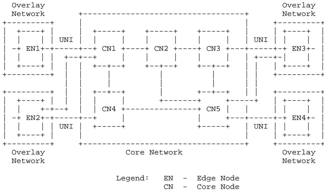
Figure 1: Overlay Reference Model [RFC4208]
