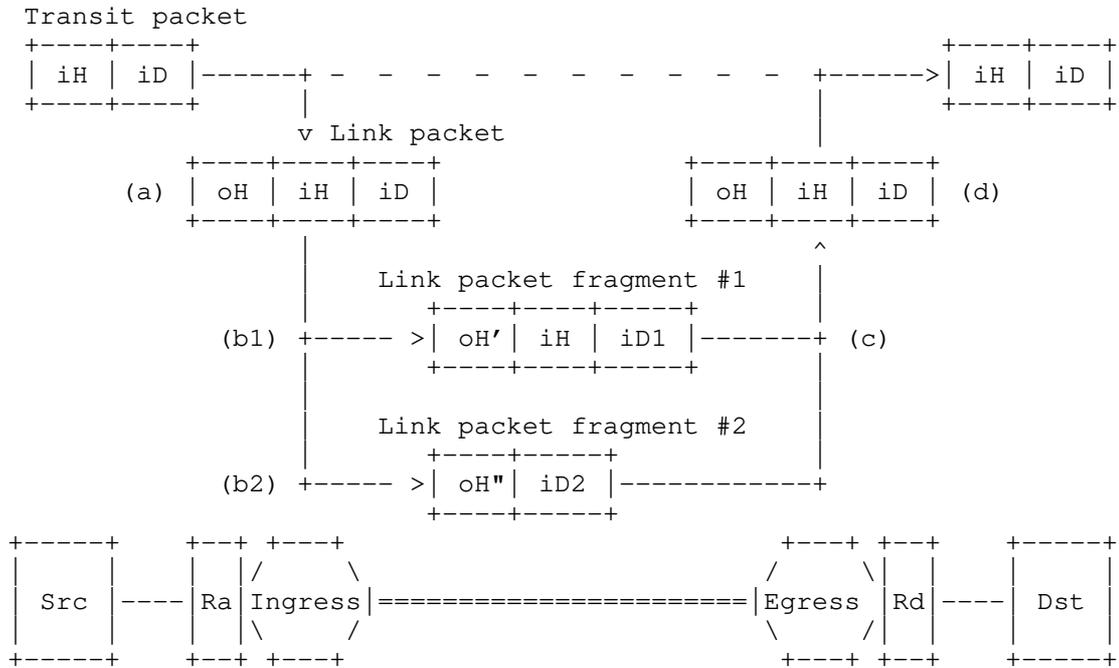
Figure 8 Fragmentation of the (outer) link packet
