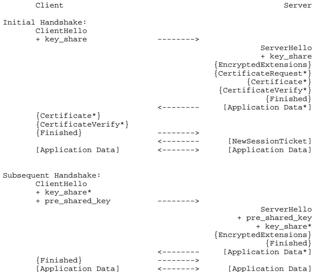
Figure 3: Message flow for resumption and PSK
