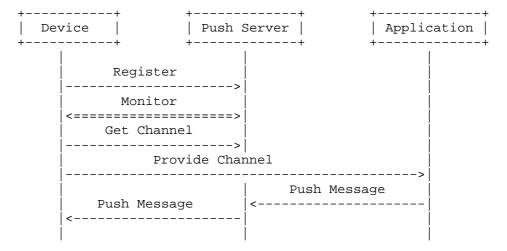
At the very beginning of the process, the device registers with the push server. This establishes a shared session between the device and push server that will be used to aggregate push messages from all applications that the device interacts with.
