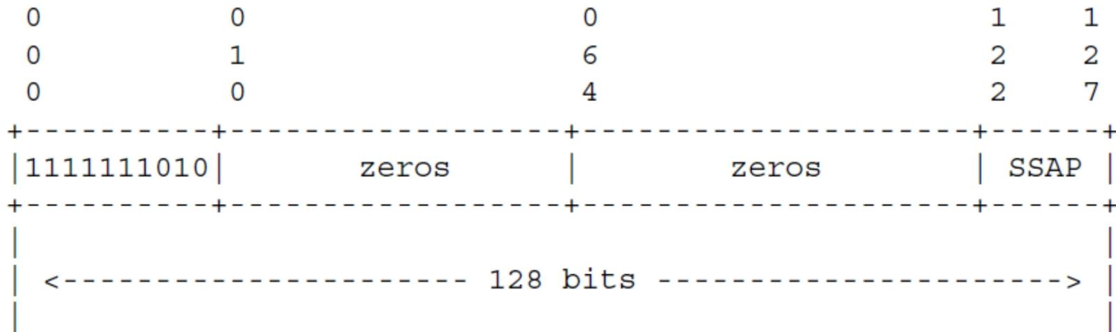
Figure 4: IPv6 link-local address in NFC
