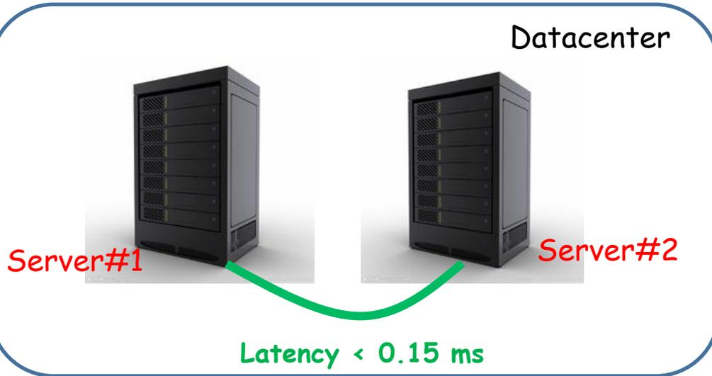
In datacenter, the latency between physical servers is relative small (**less than 0.15ms**); but in datacenter implementing virtualization, the end-to-end latency is significant, mainly for two reasons:
