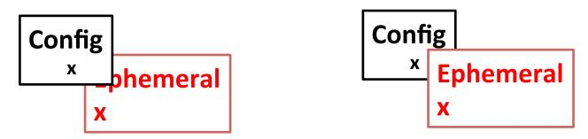
x could overlap in different datastores in the same place in the schema. Depending on "priority", a read operation on x may return either the config datastore copy or the ephemeral datastore copy.
