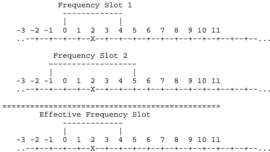
Figure 4: Effective Frequency Slot
