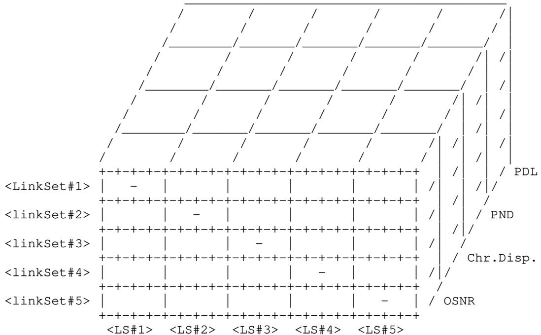
The connectivity matrix from [RFC7579] is only a two dimensional matrix, containing only binary information, through the LinkSet
