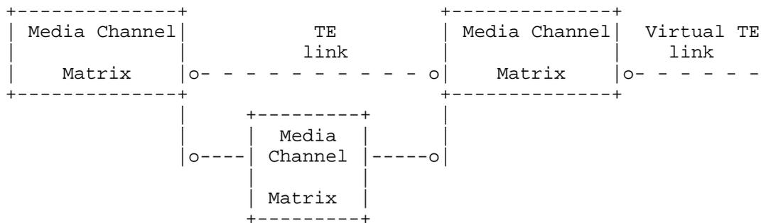
Figure 14: Topology View with TE Link / FA
