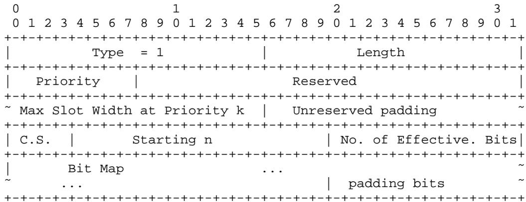
Type (16 bits): The type of this sub-TLV and is set to 1.
