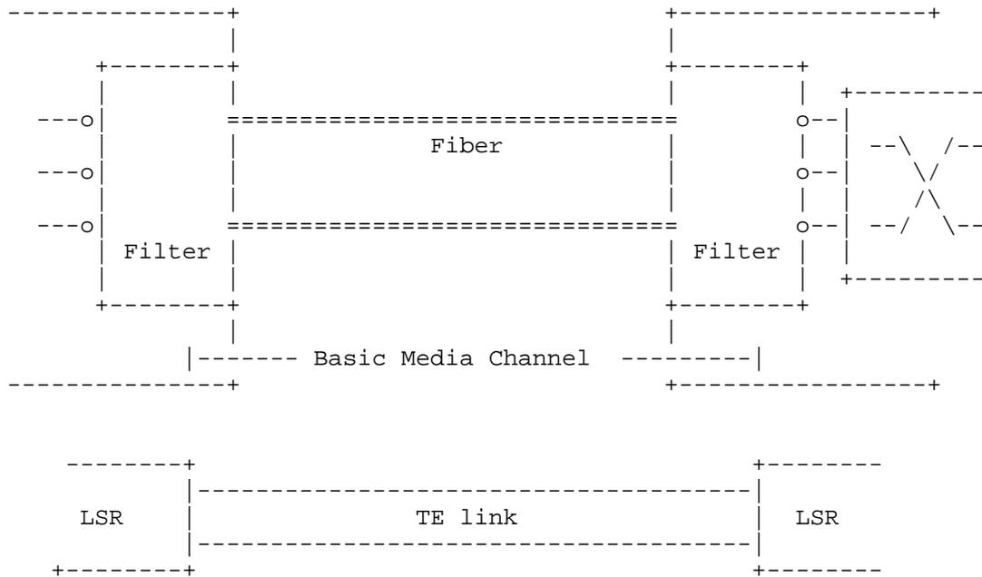
Figure 8: (Basic) Media Channel and TE Link
