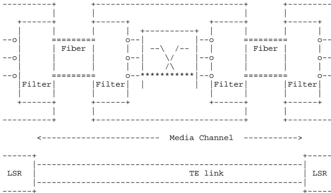
Figure 10: Extended Media Channel / TE Link / FA
