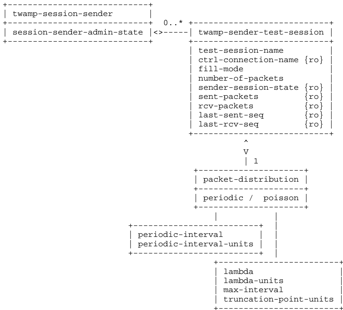
Figure 5: TWAMP Session-Sender UML class diagram
