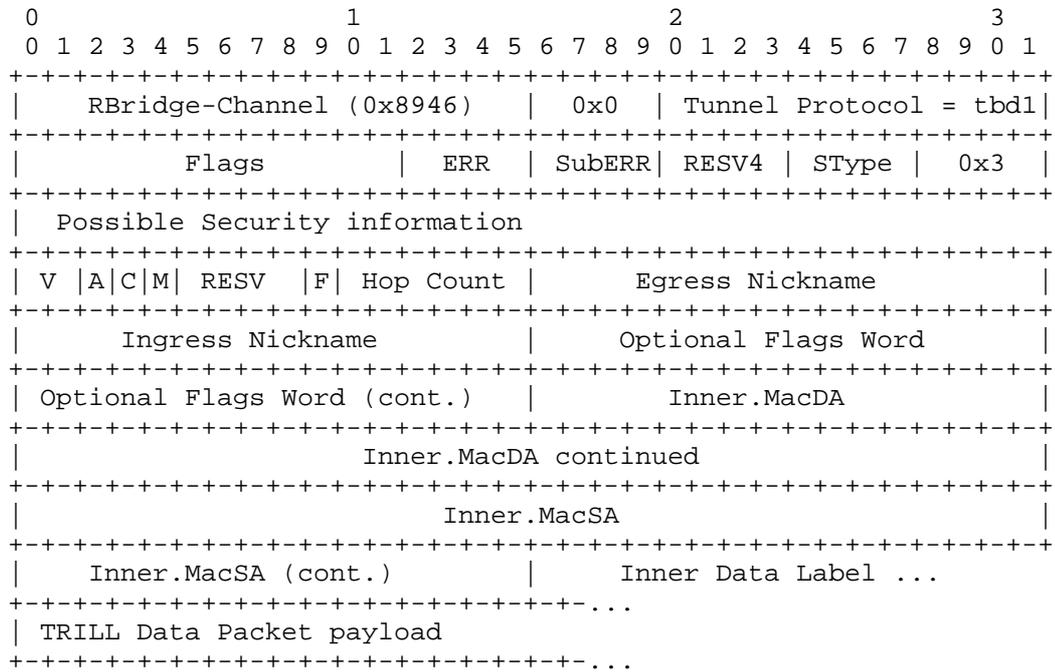
Figure 6. Nested TRILL Data Packet Channel Tunnel Structure
