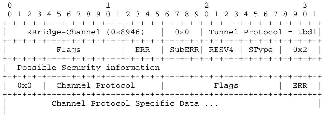
Figure 5. Tunneled Channel Message Channel Tunnel Structure
