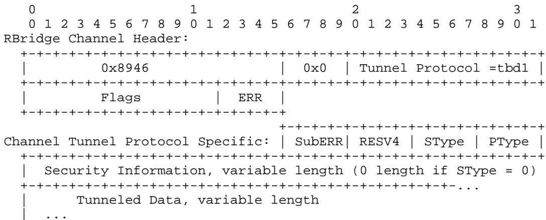
Figure 4. Channel Tunnel Header Structure
