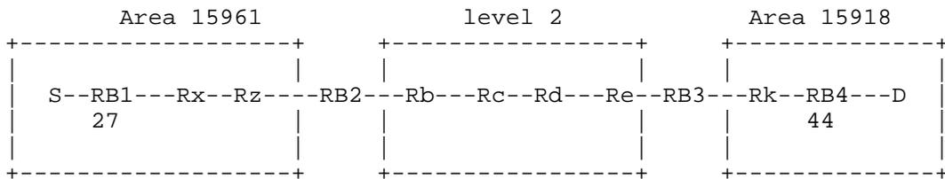
Let's say that S transmits a frame to destination D, which is connected to RB4, and let's say that D's location has already been learned by the relevant TRILL switches. These relevant switches have learned the following:
