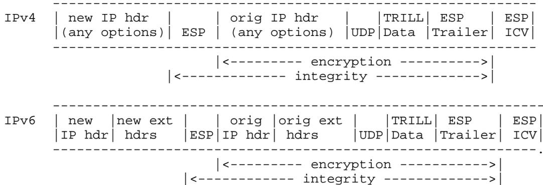
This architecture permits the ESP tunnel termination to be separated from the TRILL over IP RBridge port and, for example, placed at a physical or administrative security boundary. If two or more RBridge TRILL over IP ports are communicate securely using IPsec, there are three possibilities:
