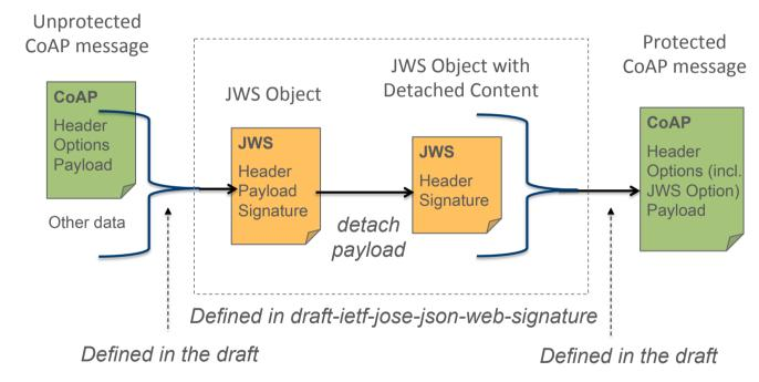
Subset of CoAP Header, Options, Payload and other data wrapped in a JWS Object
