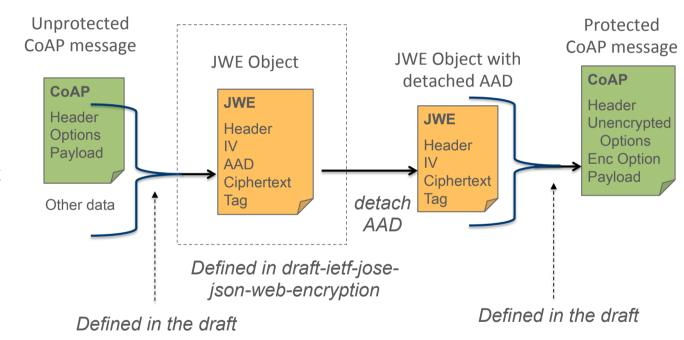
Subset of CoAP Header, Options, Payload and other data wrapped in a JWE Object
