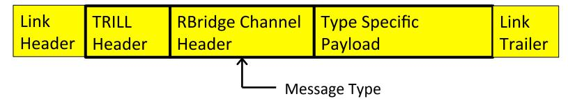
It is also useful to be able to send control messages between TRILL switches and end stations. In this case, the messages are addressed by MAC address since end stations connect by Ethernet:
