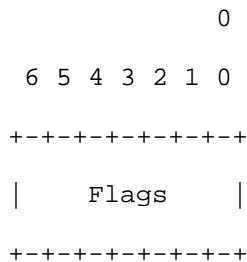
Figure 4: Block Processing Control Flags Bit Layout
