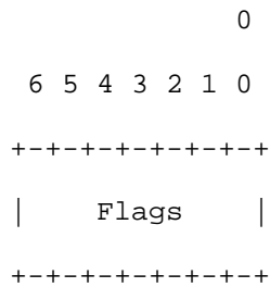
Figure 4: Block Processing Control Flags Bit Layout
