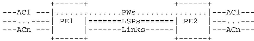
Figure 1: Explicit PW-to-LSP binding scenario
