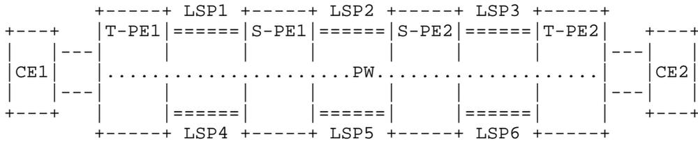
Figure 7: PSN binding operation in MS-PW environment
