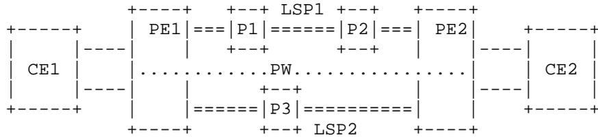
Figure 2: Inconsistent SS-PW to LSP binding scenario
