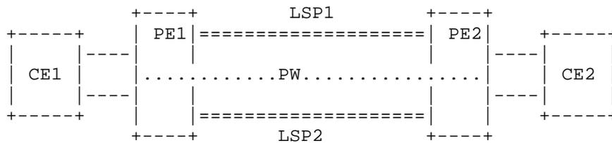
Figure 6: PSN binding operation in SS-PW environment
