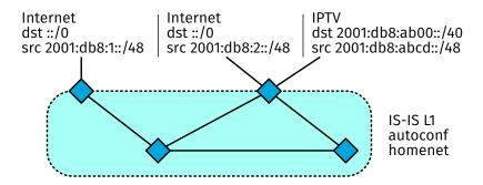
⇒ ensuring correct exit taken based on packet source address
