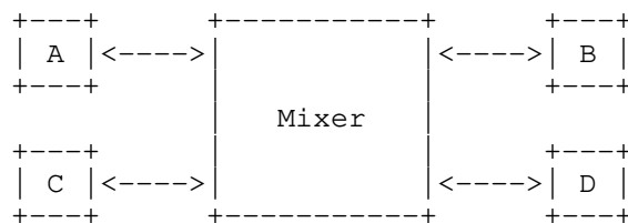
Figure 2: RTP Mixer in Unicast-only
