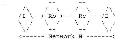
Figure 7 Tunnels, as viewed from within the tunnel
