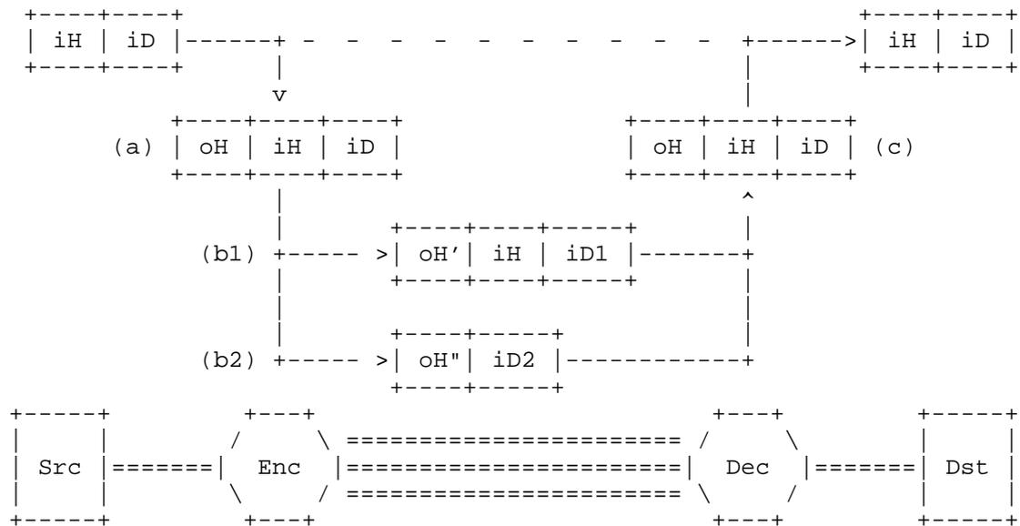
Figure 10 Fragmentation of the outer packet
