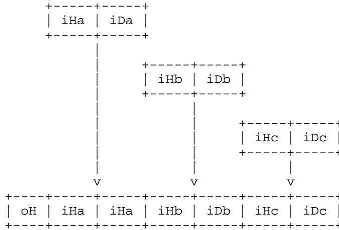
Figure 14 Packing packets into a tunnel
