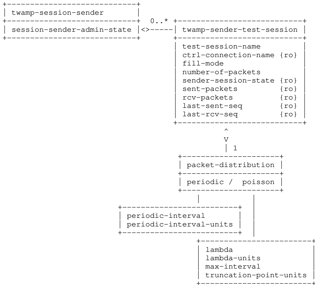
Figure 5: TWAMP Session-Sender UML class diagram
