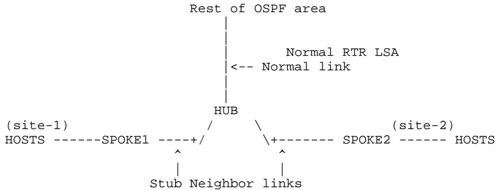
Simplified HUB Local RTR LSA contains only p2p link and a stub link with default or configured range
