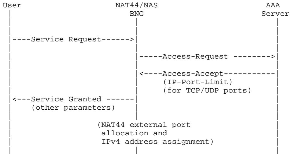
Figure 15: RADIUS Message Flow for Configuring NAT44 Port Limit
